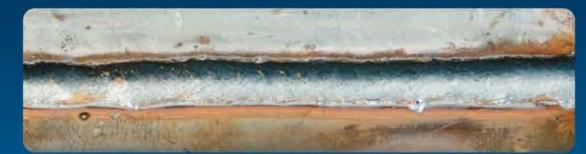
Voltage too low. Excessive spatter, poor arc control.
