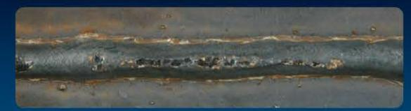
Amperage too high. Wide bead, excessive spatter, possible burn-through.
