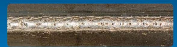
No gas. Pinholes and porosity in weld.
