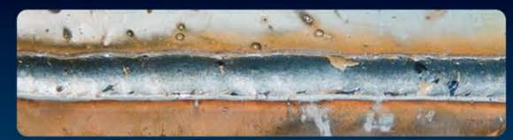
Voltage too high. Globular transfer, poor arc control.
