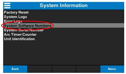
29. The <u>System Software Numbers</u> window will open and display the software revision for each printed circuit board and the overall system software. If the displayed software revisions match the downloaded software revisions, the machine software has been successfully updated.
