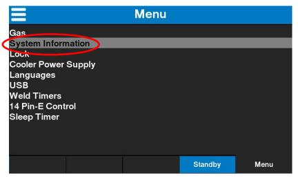
28. The <u>System Information</u> window will open. Rotate the control knob to the <u>System Software Numbers</u> option and push the control knob in to select option.
