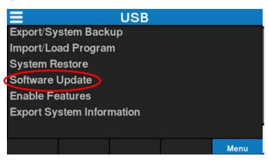
25. After the <u>Software Update</u> option has been selected, the screen will display "System Software Update in Process DO NOT remove power." Do not remove power during the update process.
