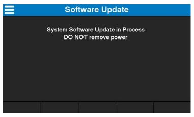
26. The screen will display "System Software update done Please cycle power" after the software update is done. Remove the USB Flash Drive from the machine and turn the machine off. Wait for the fan motor to stop spinning before turning on the machine on. Upon power up, the machine will apply the software updates. This may take a few seconds to several seconds.
