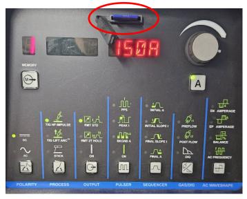
23. The LED below the SD card port will *flash* **green** to indicate it is updating. Do not remove the <u>SD card</u> or power from the machine during software update process. After the software update is complete, the LED will turn *solid* **green**, and the <u>SD card</u> can be removed from the machine.
