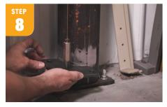
Before welding the bottom base plate, grab your plumb bob and drop it through the hole in the top base plate to ensure the pivot points will line up on both base plates. Make your mark and drill a 5/8" hole. Then, weld the bottom base plate to the vertical post.
