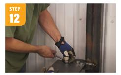
With the mounting base extended out, transfer punch the top holes to the top base plate, drill and tap for your 1/2" locking bolts.
