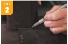
Use a template to draw a line to cut notches out of the top and bottom base plates so they can be welded to the vertical post.
