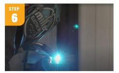
Using the Millermatic 255, tack weld the top base plate to the vertical post. Using pulse MIG mode, I set the machine for 3/8"-thick material with Auto-Set™ technology.
