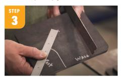
Measure the pivot point of the top base plate, which will be welded to the post. This will enable the stand to swing around the post. Mine is 2-3/8" away from the corner. That gives me 1-3/8" clearance to work with for the mounting base. Keep in mind you also have to put a weld on the top base plate and it will take up at least 1/4". Follow the same directions for the bottom base plate.
