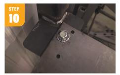
Machine your 5/8" hole 1" from the end and 2" from the side in your mounting base along with two 1/2" holes, which will be used for your locking bolts. The locking bolts will be tapped into the swivel mounting base once the table is fully extended.
