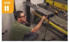
After attaching both the bottom swivel plate and mounting base with your 5/8" bolts, place your digital level on the mounting base and shim it up until it's perfectly level. Then measure for your diagonal support tube that will go from the end of the mounting base to the bottom swivel plate and weld it into place.
